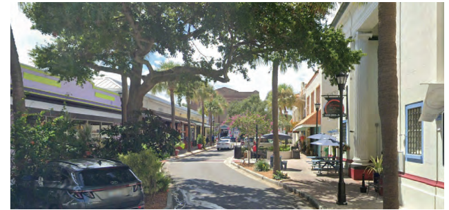
Offset curb extensions on Harrison Street have helped to create more pedestrian friendly connections
