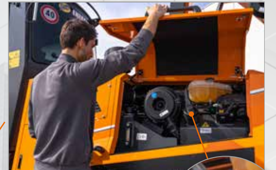
DIESEL AND OIL SUPPLY COMPARTMENT AND FILTER MAINTENANCE
