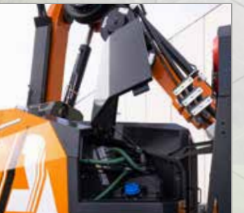
DEF SUPPLY COMPARTMENT
